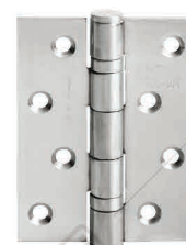
ESS DL 4X3X3MM 2BB SSS Capacity (max) : 75 KG / pair
